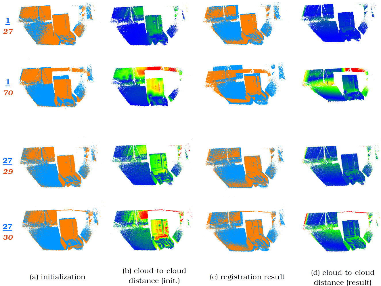
Figure VI: Results of the experiment on the CoRBS dataset [7]: (a) initial misalignments (initialization); (b) cloud-to-cloud distance corresponding to the initial misalignment; references are shown in cyan and templates in orange; on the left, corresponding frame numbers are provided (in cyan for the reference frames and in orange for the template frames). (c) GA registration results; (d) cloud-to-cloud distance corresponding to the registration result; cloud-to-cloud distances are coded with a Blue<Green<Yellow<Red color scale; the saturation point (red value) amounts to 0.1 distance units.
